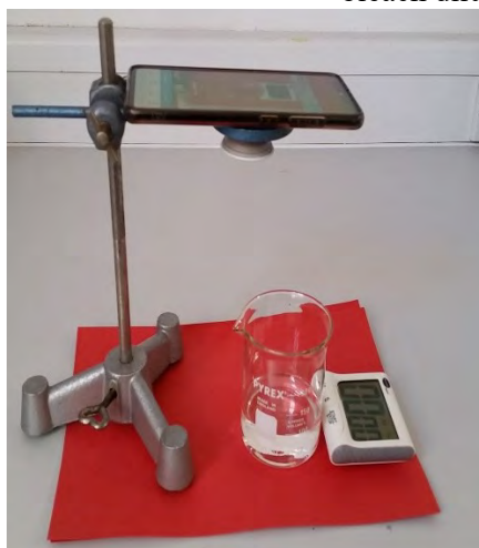
Figure 3: Set up for experiment; (a) materials required; (b) set up of camera, reaction flask and times; (c) camera view with RGB app.
